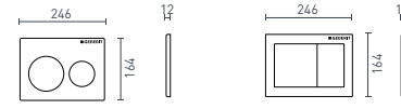
ROUND BUTTONS (p. 6) 246 x 12 x 164 mm SQUARE BUTTONS (p. 6) 246 x 12 x 164 mm
