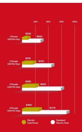
Estimation based on EHPA250VMA STC's in Zone 3 under medium load, obtained rom independent laboratory test results and followed by TRNSYS modelling and a etail electricity cost of \$0.30c per kWh.
